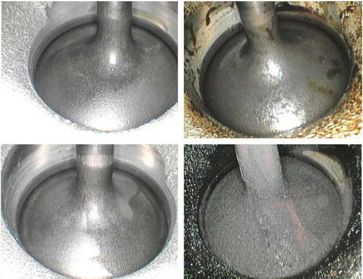
Side-by-side Gunk Comparisons. Top Row: Intake valves before and after running Shell's V-Power NiTRO+; Bottom Row: Intake valves before and after running on a competitor's premium gasoline. Images courtesy of Shell
